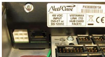
*RJ-45 Link Connector on the rear panel*
