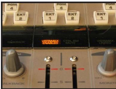
**The VistaMax Enabled Label lights on the Monitor Control Panel when the Link is Activated**
