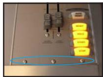
**M3x6 Panel Screws (two on Dual Faders, three on the Monitor Control panel)**
