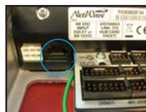
**The RJ-45 Link Connector on the back panel**
