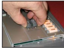
**Lightly squeeze the fader knobs together to lift a control panel out of the chassis**
